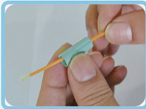
Put the cable into the boot 1.1 光缆穿入尾套
