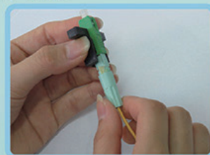
Unlock the boot, Put out the fiber 3.3 解开螺尾套, 取出光纤
