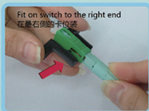
Assemble the auxiliary jig 3.1 装助推块
