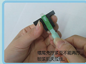
Lock the boot 2.3 拧紧螺尾套
