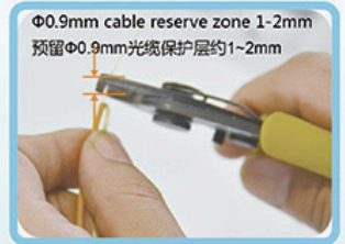
Strip the \Phi 0.9 mm cable cover 1.4 剥去 \Phi 0.9 mm光缆保护层
